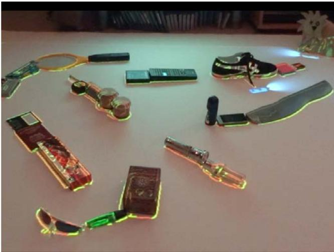
Fig. 2. Outlines showing the system's real-time obstacle detection. In the upper right corner: 'Green player' is stuck inside an object and can only be freed by moving it.
